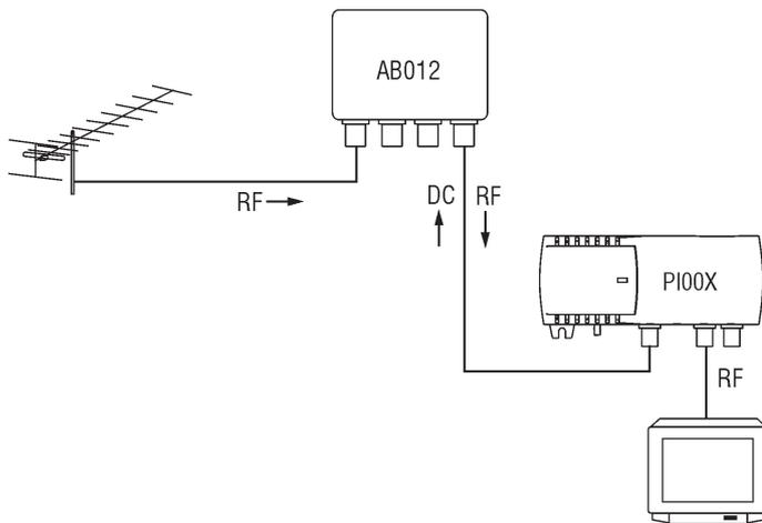
2. Application diagram using other power supplies 4.5 V ÷ 12 V 100 mA max., connected together with power inserter.
